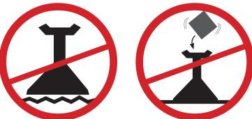
Safety Stands are capacity rated to static loads. Shock loads could weaken, damage or destroy the stands. Shock loads include dropping the load onto the stand or ground tremors due to blasting or nearby heavy equipment moving. In this case, additional support should be used.
