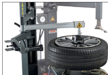
Positions the rim during locking operation
