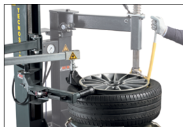
Maintains the tire bead on the rim facilitating the demounting procedure
