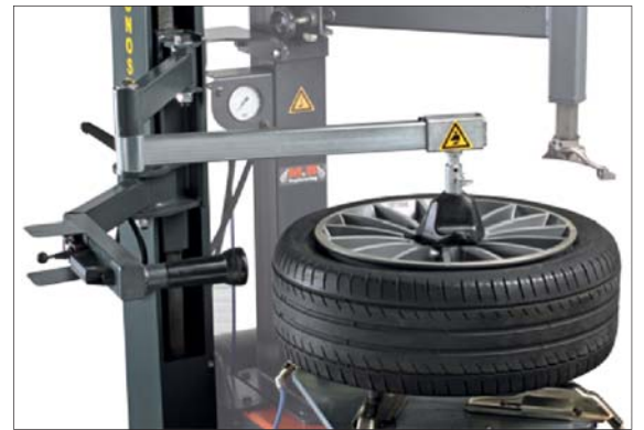
Positions the rim during locking operation
