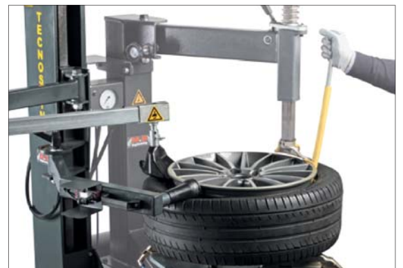
Maintains the tire bead on the rim facilitating the demounting procedure
