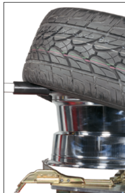
Roller arm with the option of operating under the tire greatly helps in the demounting and mounting
