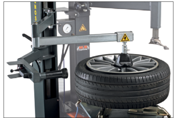
Positions the rim during locking operation
