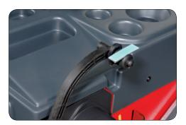
Alu data program that resolves all the problems of balancing aluminium rims. The arm in the central part of the weight holder panel indicates the exact position for application of adhesive weights.
