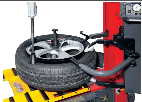
In addition to upper and lower Bead Breaker roller arm, Power Assist Roller Arm provided to simplify mount operations and Mobile bead depresser helper arm follows the rotation of the tire
