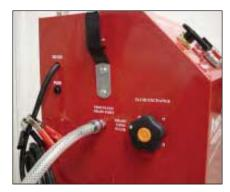
Simple evacuation port and valving for pumping used transmission fluid into bulk storage The transmission **POWER FLISH** is fast and easy to use. The Optional DeSludge process cleans the entire Transmission in less than 10 minutes
